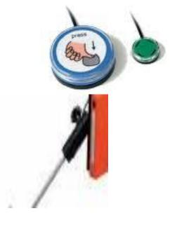
The **Switch Hopper** provides an interface allowing you to plug switches into a computer. When you plug a switch into one of the three Switch Hopper jacks, it mimics mouse-clicks, and with the installation of the accompanying software, you can configure each button to be any mouse-button event.
